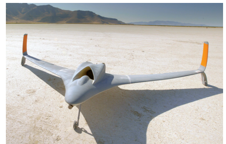
Final 3D printed jet-powered aircraft.
