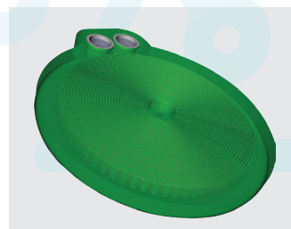
CAD model of electromagnet 3D printed coil
