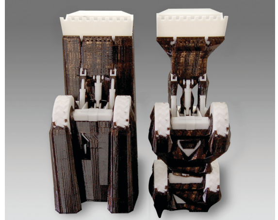
Figure 2 - A toy tractor model (white) with support material (brown) still attached.
