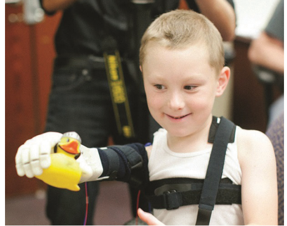
Figure 11 – Alex tries out his 3D printed bionic arm made with FDM technology.
