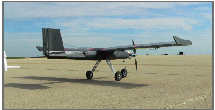
SelectTech chose FDM technology to avoid tooling headaches with this UAS with an all-FDM airframe.
